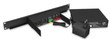
The green multi-connector consists of two parts. On the left-hand side, we find the tri polar part for connection to the remote control. On this connector a wire bridge is assembled between 1 and 2. Only remove this bridge when a remote control is connected.
