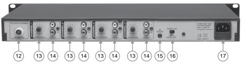
12. FM Antenna. This socket has to be used to connect your 75 ohms FM antenna. You can use the shipped indoor "wire" antenna, but to improve the reception, we advise to install an outdoor FM antenna or to connect the PR4000 to a cable radio network. Normally, when you use a cable radio network you must use a ground isolator transformer adaptor (GIT). Since your PR4000 is already equipped with a build-in GIT, it is not necessary anymore to use or to buy such an external transformer.
